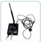
The Industrial Router connects the equipment with the internet. It features a Wi-Fi access point and a 3G modem. It can be managed via SMS and keeps itself alive while bad connections. In combination with the Communication Module the router allows the equipment to activate functions like status e-mails, event e-mails, web interface and file transfers. The router will be pre-configured ready to use – only a SIM card with a flat rate is needed.
