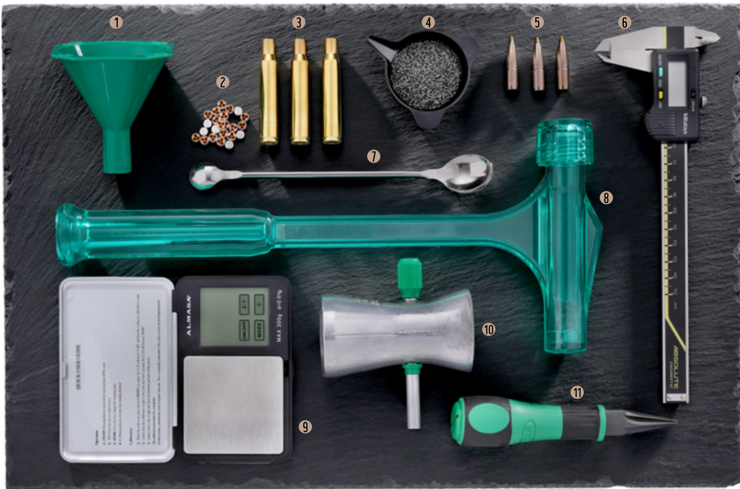
1 – Powder funnel, 2 - Primer, 3 – Cartridge case, 4 – Powder scale pan, 5 - Bullet, 6 - Digital caliper, 7 – Laboratory spoon, 8 – Kinetic bullet puller, 9 – Digital powder scale, 10 – Powder trickler, 11 – Case mouth chamfering tool
